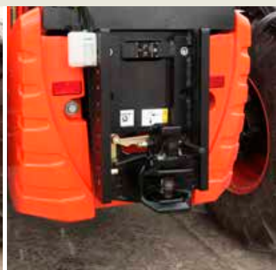
Rotating tow hitch with height adjustment
