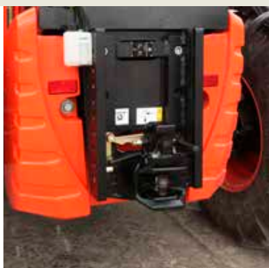
Rotating tow hitch with height adjustment
