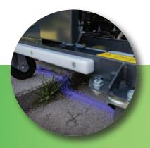
The sensor sparys water only where it detects chlorophyll. This keeps water usage, emission and fule consumption to a minimum, resulting in the lowest cost pr. treated m² comapred to any other non-chemical weed control machine on market.
