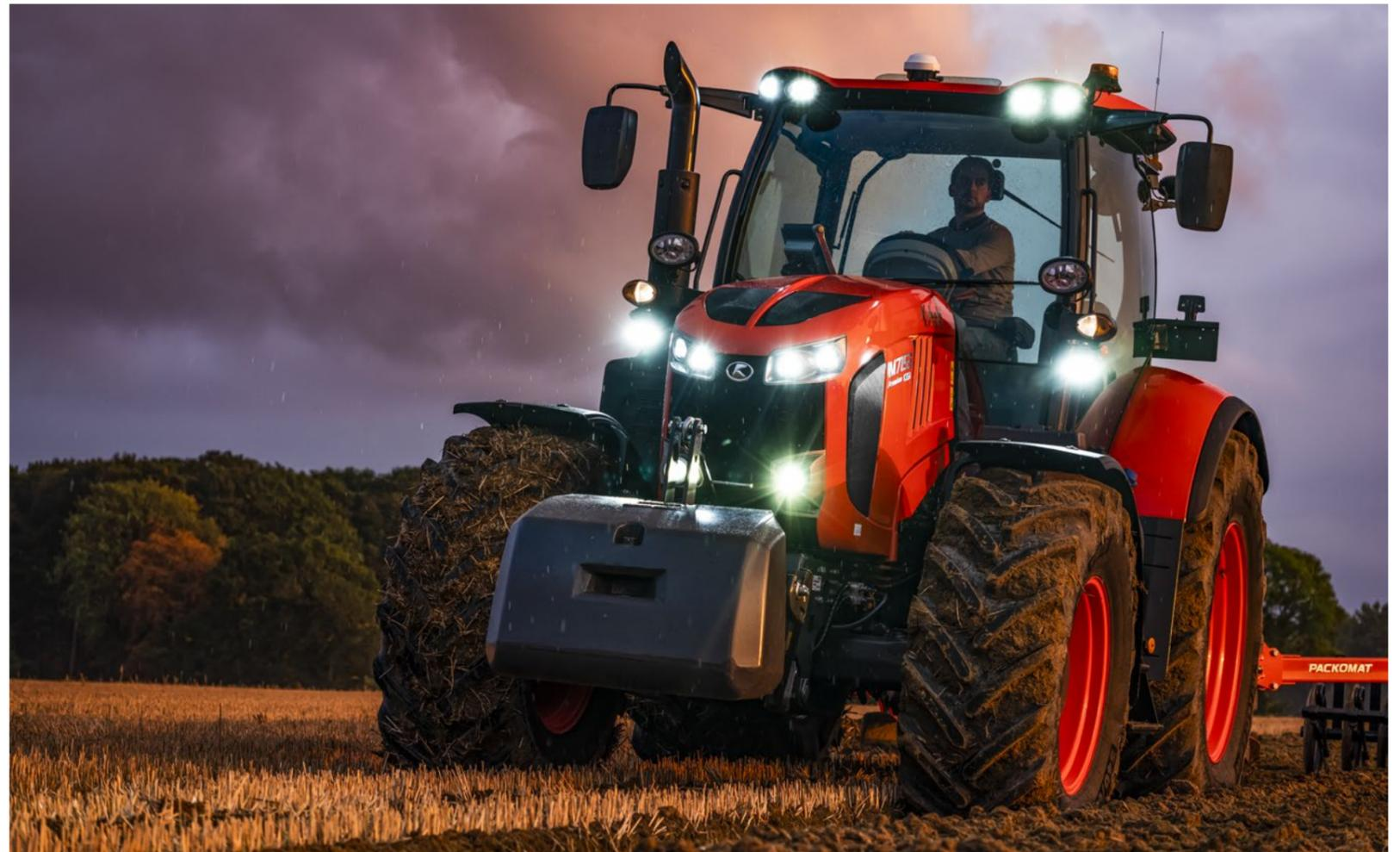
Front axle and cab suspension protect both operator and machine and result in high productivity. Relative to front axle: With the heavy duty version, the M7003 is equipped with an extremely robust front axle. The tractor is available without cab suspension or can be equipped with two different suspension systems: a mechanical suspension system or a pneumatic suspension.
