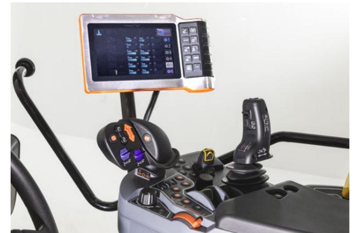
With the Kubota M7003 you can optionally integrate all control elements into the modern arm rest. All the controls you need on a regular basis are within easy reach without having to lift your arm. This means even more comfort and productivity for you – intuitive operation included.
