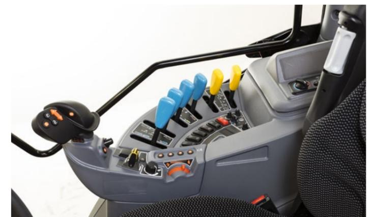
On all M7003 models, some additional controls are centrally located on the right side. The multi-function lever on the standard model is integrated into the side console, while the higher models are equipped with a modern armrest and multi-function lever.
