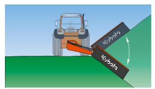
Kubota DM2000 series can pivot  $35^{\circ}$  up and down without any adjustment.
