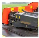
The auger is driven by a small gearbox with an additional power requirement of only 5hp.
