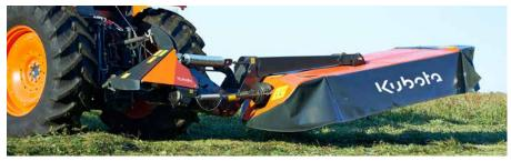
Lifting on headlands via hydraulic cylinder - ample ground clearance.
