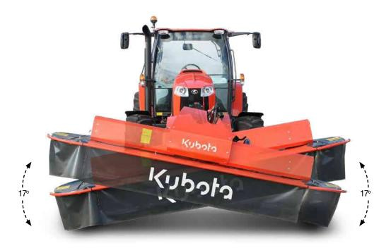
The mowing unit moves independently from the front linkage, ensuring the best possible pattern of movement and the transverse adaptation sets the standard in this segment.
