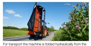
tractor cab to the vertical transport position well behind the tractor, ensuring a stable and steady transport.
