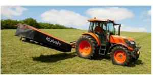
Lift on headlands via a hydraulic cylinder – no use of the 3-pt hitch is needed.
