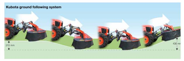
An adaptation range of 430mm upwards and 210mm downwards ensures untroubled ground following.
