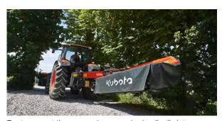
For transport the mower is swung hydraulically into horizontal position behind the tractor. Fast and easy conversion, with no need to leave the tractor.
