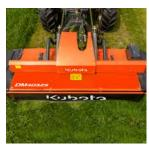
Two speed driveline is standard. Standard speed is 1000 rpm. By switching driveline pulleys 750 rpm, for reduced fuel consumption, is possible.
