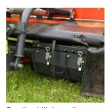
Swath width is easily changed by simply unlocking the swath plates and sliding them to the requested position.
