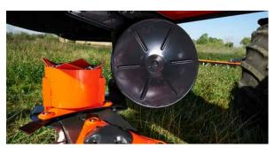
The machine is standard equipped with two swath discs, allowing a swath width of 2.2-2.4m.
