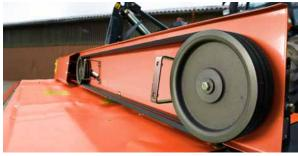
By switching driveline pulleys changing from standard PTO speed of 1000 rpm to 750 rpm is possible.
