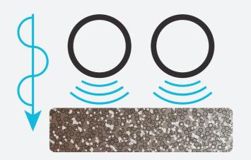
0.5 mm amplitude for sub-structure applications
