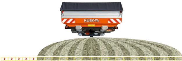
Decreasing the spreading width on the left hand side by 10m
