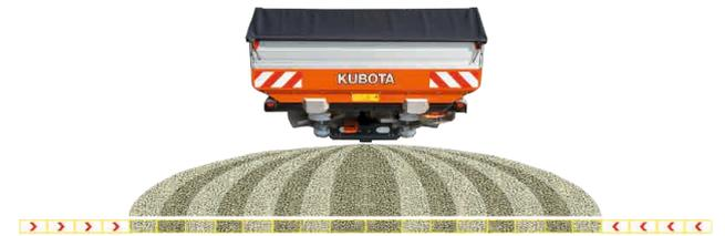
Decreasing the spreading width on both sides by 8m
