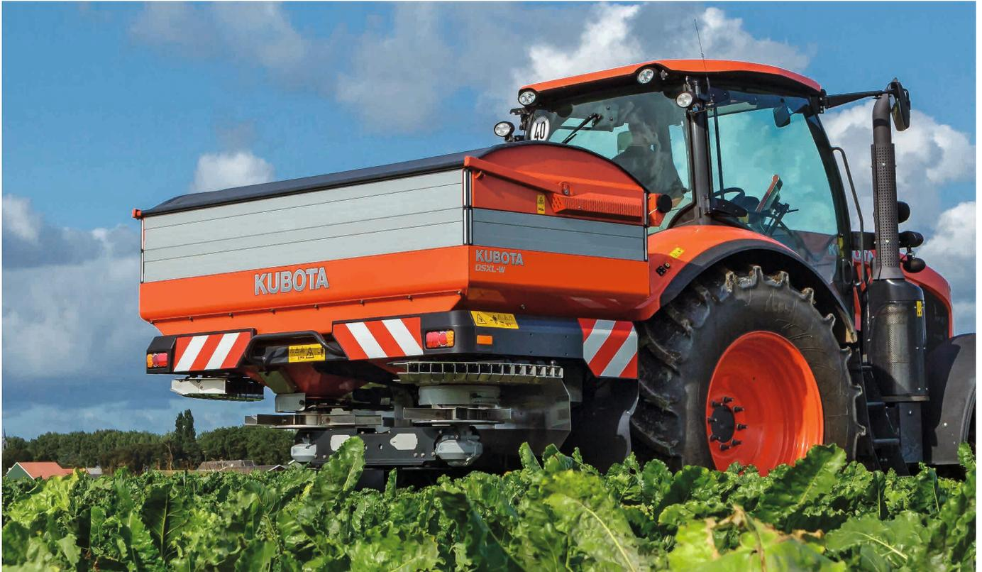
The DSM-W and DSX-W are weighing spreaders with the advantage of speed related spreading and high frequency automatic calibration. The DSM-W has hopper volumes from 1,100 - 2,000 litres, can spread up to 28 metres and has one 10 tonne load cell. The larger DSX-W has more capacity with 1,500 - 2,800 litre hopper volumes, can spread up to 54 metres and it has four 5 tonne load cells positioned on both the front and the rear side of the spreader for the most accurate weighing.
