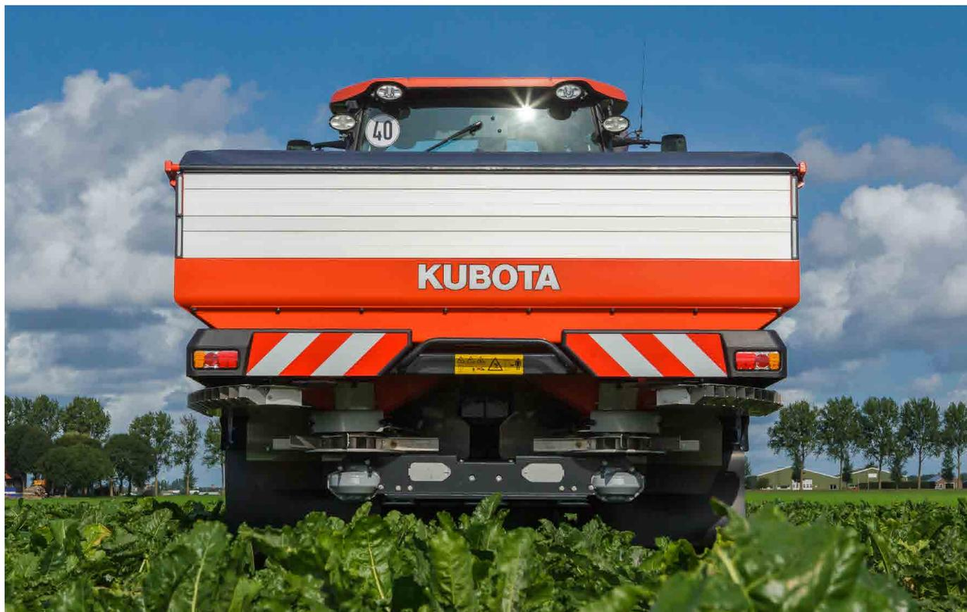
A border spreading device is used to optimise your spreading pattern from or to the border of a field. With the result of a maximum coverage to the border of the field to ensure a good crop, while on the other hand a minimal loss over the field border to minimise environmental impact.
