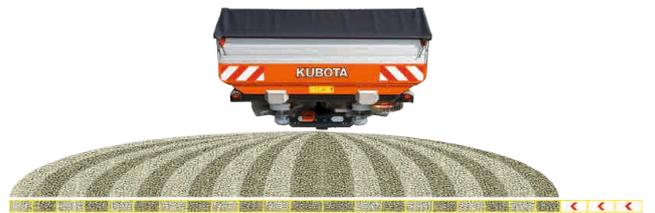
Decreasing the spreading width on the right hand side by 6m
