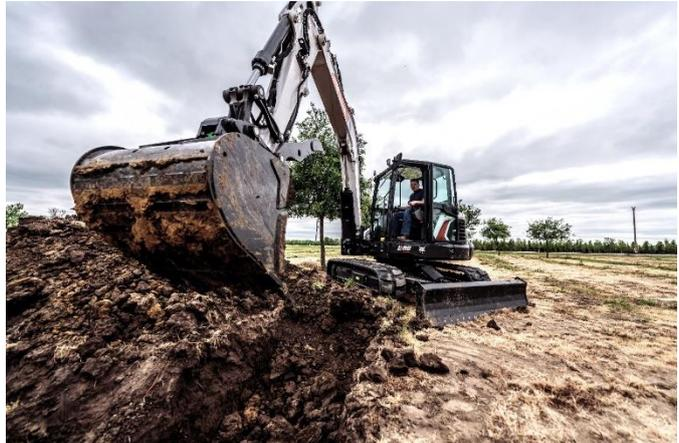
components, as well as all the hoses, pipes, valves, lights and other sensitive components that are important for excavator functions. The design of the machine also eliminates the 'unicorn effect' of having the boom swing cylinder exposed during offset parallel digging, reducing the risk of damage to the surroundings and the cylinder itself.
