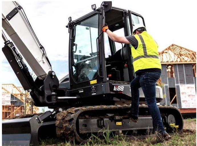
Easy and safe to step in and step out thanks to the wide doors, unique 3D handle, anti-slip step on the undercarriage and foot space above the track, the cab makes the daily life of the operator an easier one.
