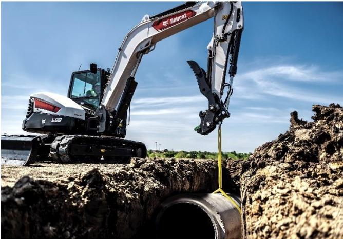
R2-series machines are designed to achieve superior 360-degree stability in any situation, even when digging over the side or when handling heavier loads. They are well-balanced machines for operating with different attachments owing to improved weight distribution, extended track length, optimized counterweight design and dual flange rollers guaranteeing superb over the side stability. This assures operators of confidence in any situation, even without
