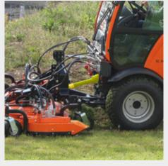
**Mechanical PTO shaft (not B 55)** Ensures constant power transmission to your attachments to tackle even the most heavy-duty applications.
