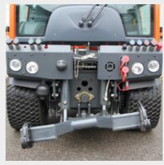
**3D front power lift** The front power lift can be adjusted 3-dimensionally to tackle any surface, no matter how uneven it is.
