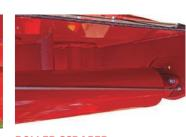
**ROLLER SCRAPER** Cleans roller and reduces clumping in wet conditions.
