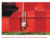
PRECISE HEIGHT ADJUSTMENT Clearly displayed indicators in both metric and imperial units and a high-tensile 2mm pitch adjuster for precise cut height alterations
