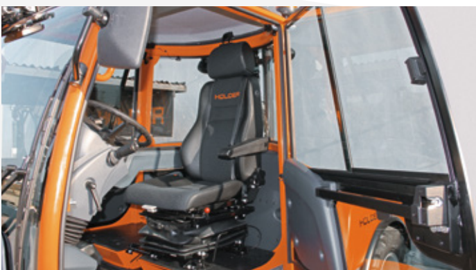
Air-suspension seat with seat heating and armrest
