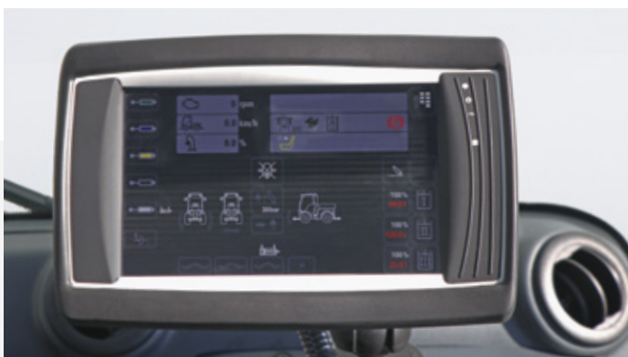
Touch display for operating all hydraulic functions
