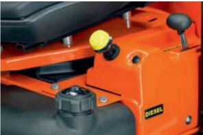
**PTO engagement switch** directly engages hydraulic drive to the front deck. No replacing or tensioning of belts, no greasing the cardan shaft or other maintenance within this area.
