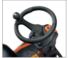
Adjustable soft-grip steering wheel Fore/aft steering wheel adjustment and steering drive knob further adds to the overall driving comfort.
