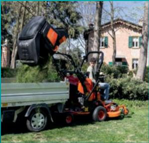
**480 litres collector**A high lift grass collector ensures you can tip the grass into a waiting trailer or on top of an existing pile. Single lever operation of the raise/lower and tip. When the collector is fully raised, continuing to operate the lever allows the tip procedure.
