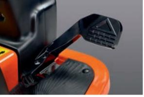
Rocker pedal drive control could not be easier. Simply press the forward part of the pedal and the HST transmission will take you to your required speed. Infinitely variable speeds are available up to 10 km/h. For reverse use the rear portion of the pedal. The smoothness and reaction of the transmission allows you to alter your speed to suit the varying ground conditions.
